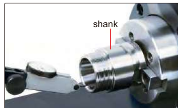
measure radial runout of shank
