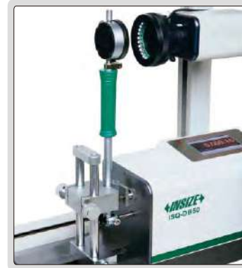
check bore gages
