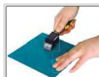
step 1: make grid cutting on surface
