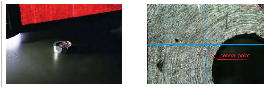
laser indicator locates the central point
