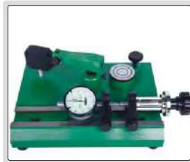
inspect accuracy of dial indicators (range 0-25mm)
