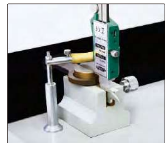
lapping measuring surfaces of caliper lower jaws
