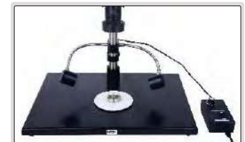
illumination direction and brightness are adjustable
