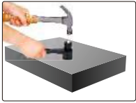
hammer impact to apply test force
