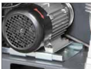
Tensionador da correia. Belt tensioner skid adjusts the tension of the belt.
